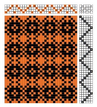
weave, but itself a treadling method. As in waffle weave, the popcorn treadling method has long floats. The name is derived from popcorn which the formed cells resemble.
